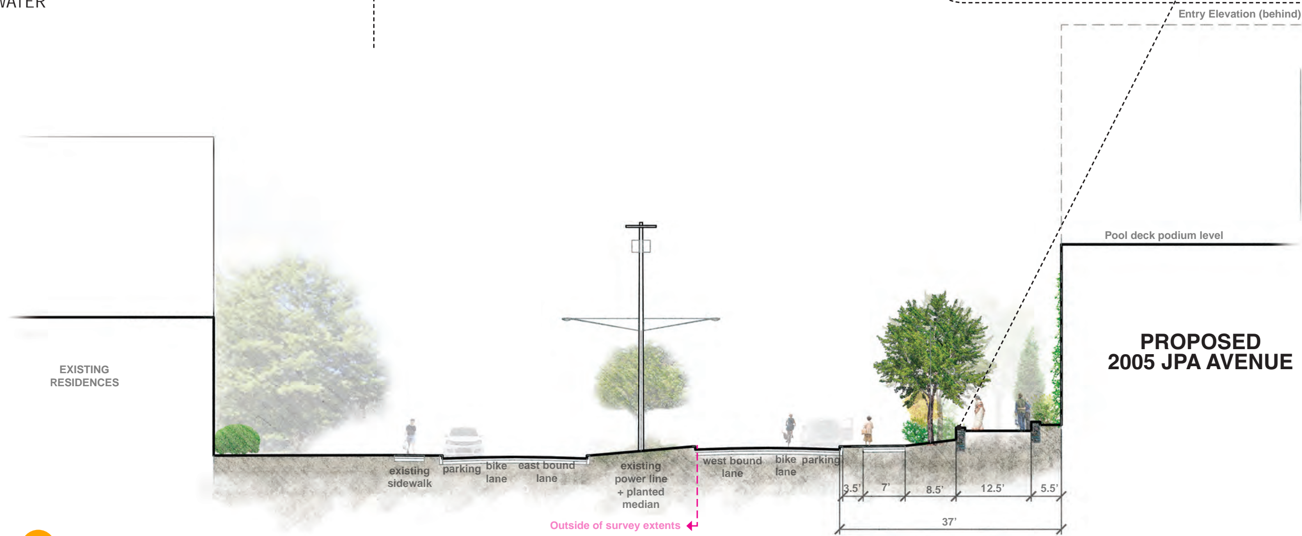
STORMWATER CONCEPT: MICRO-BIOFILTERS ALONG OBSERVATORY AVE.; NATIVE PLANTING AND WEIR WALLS/ TIERS TO SLOW THE MOVEMENT OF WATER
